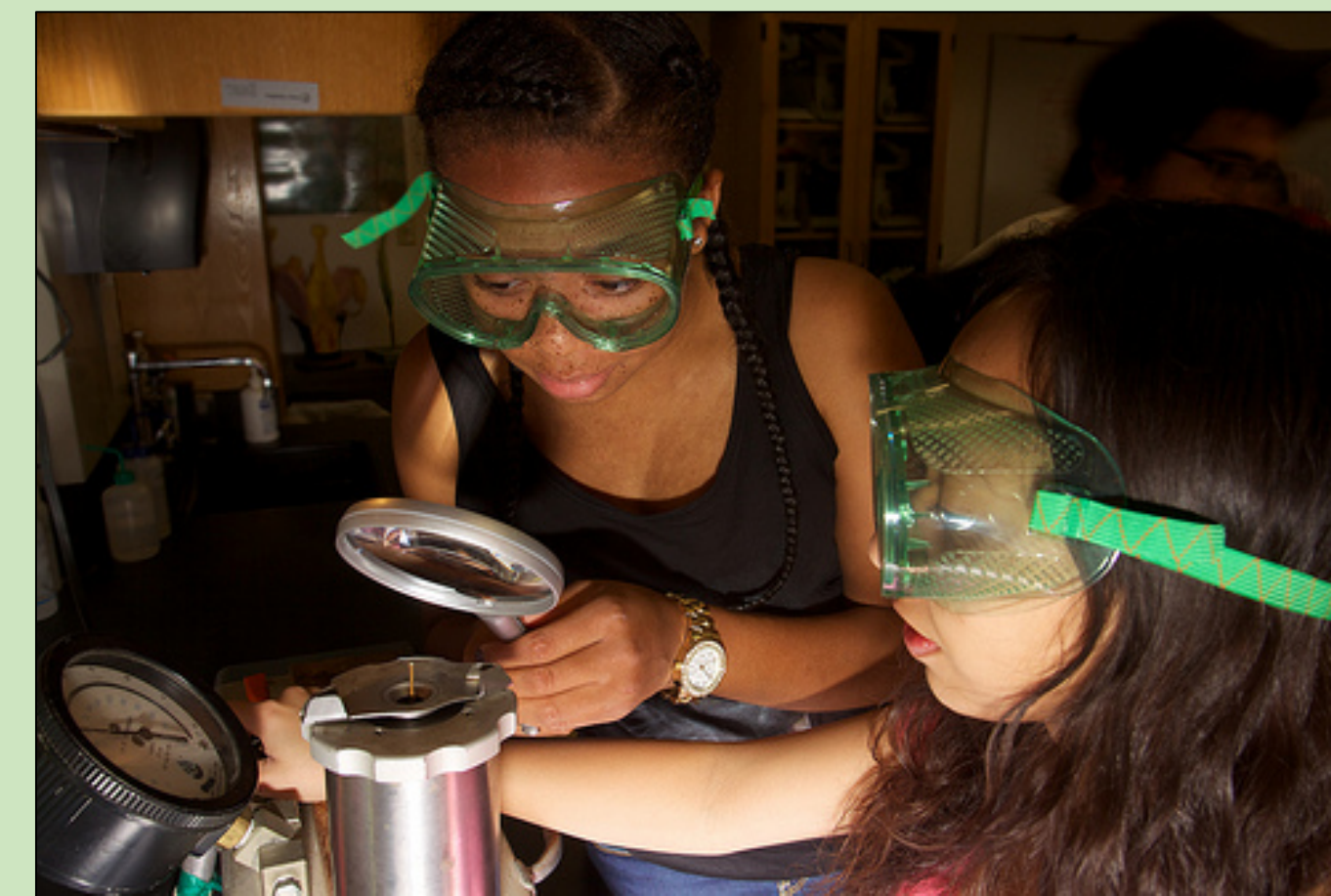
Figure 1. Data was collected by using the Scholander Hammel pressure chamber to measure the pressure inside the leaf before it was cut from the original shrub oak.
