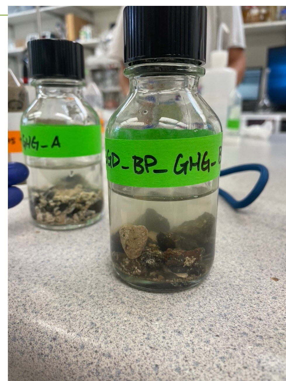
Fig 1 shows sediment and water samples of a known mass and volume in GHG incubation bottles in which 6 samples were taken from each of the two sites
