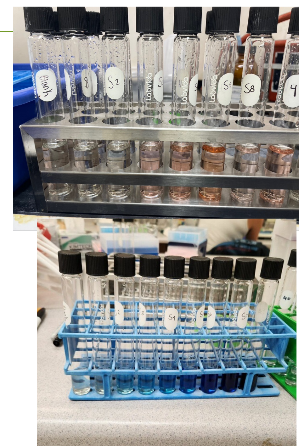
Fig 2 is an image taken from the nitrate concentration determination and Fig 3 from the phosphate determination by visible light spectrophotometer where color intensity corresponds to nutrient concentration
