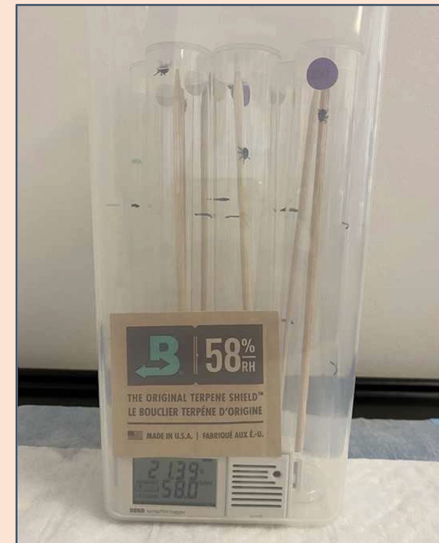
Figure 1: Airtight bin filled with tubes, skewers, ticks, RH packet, and a HOBO temp/RH logger. Photo from Kim et al. 2022
