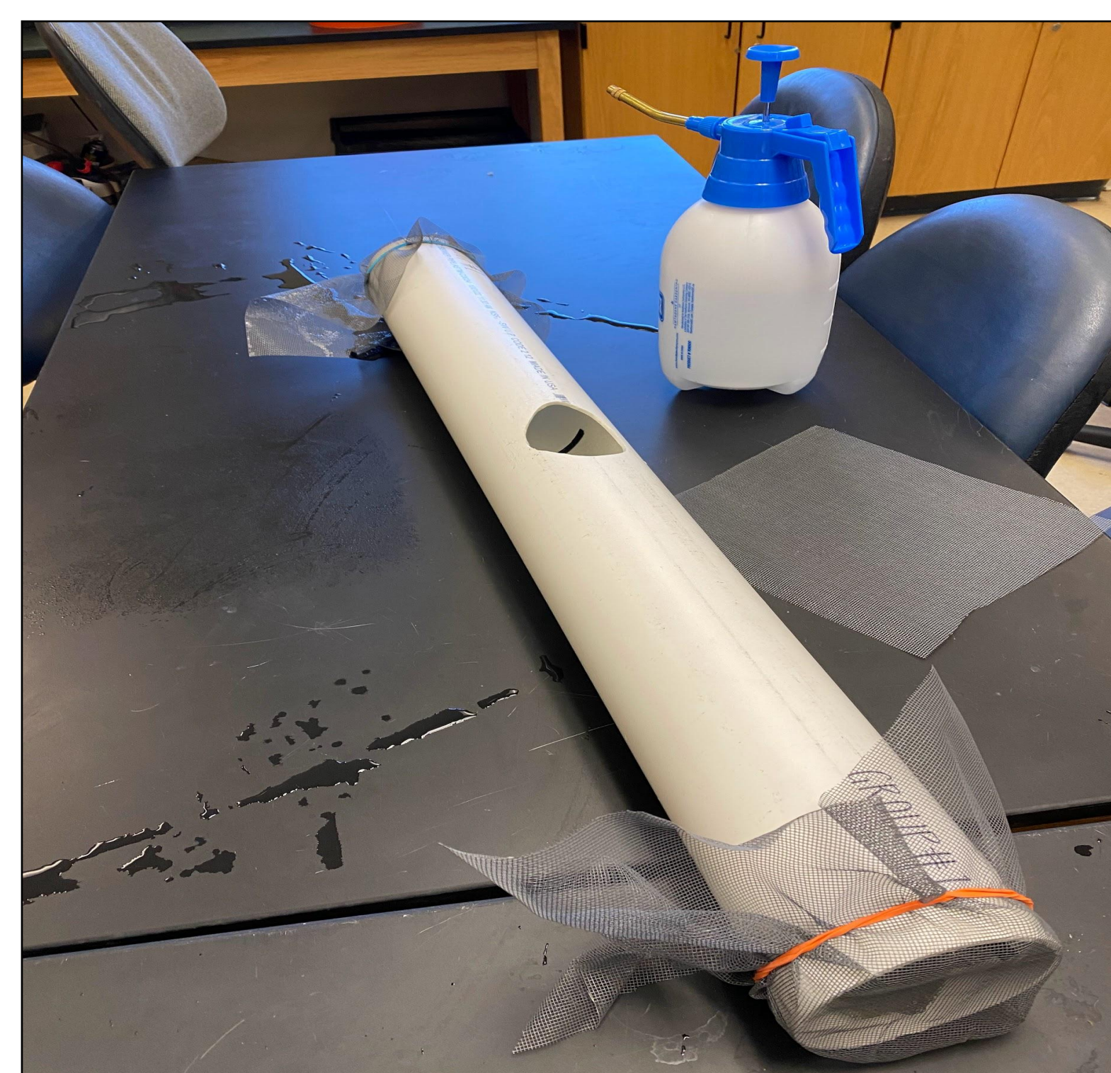
Image 2: Experimental setup of the plastic pipe with the fine wire mesh covering up the openings. A jug of carbon filtered water was used to rinse out the tubes.
