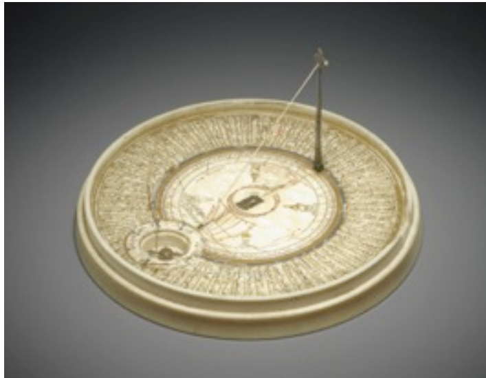
Figure 1. Bayram ibn Ilyas, Sundial / Compass / Qibla pointer , 1582-3, Ottoman Turkey. Metal, ivory, gold, fibre, and brass, diameter 11cm, height 5.5cm with metal strut unfolded. British Museum, London. www.britishmuseum.org .
