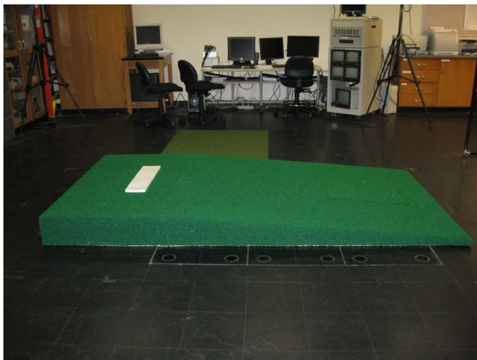
Figure 5. Pitching mound installed over Kistler force plates.
