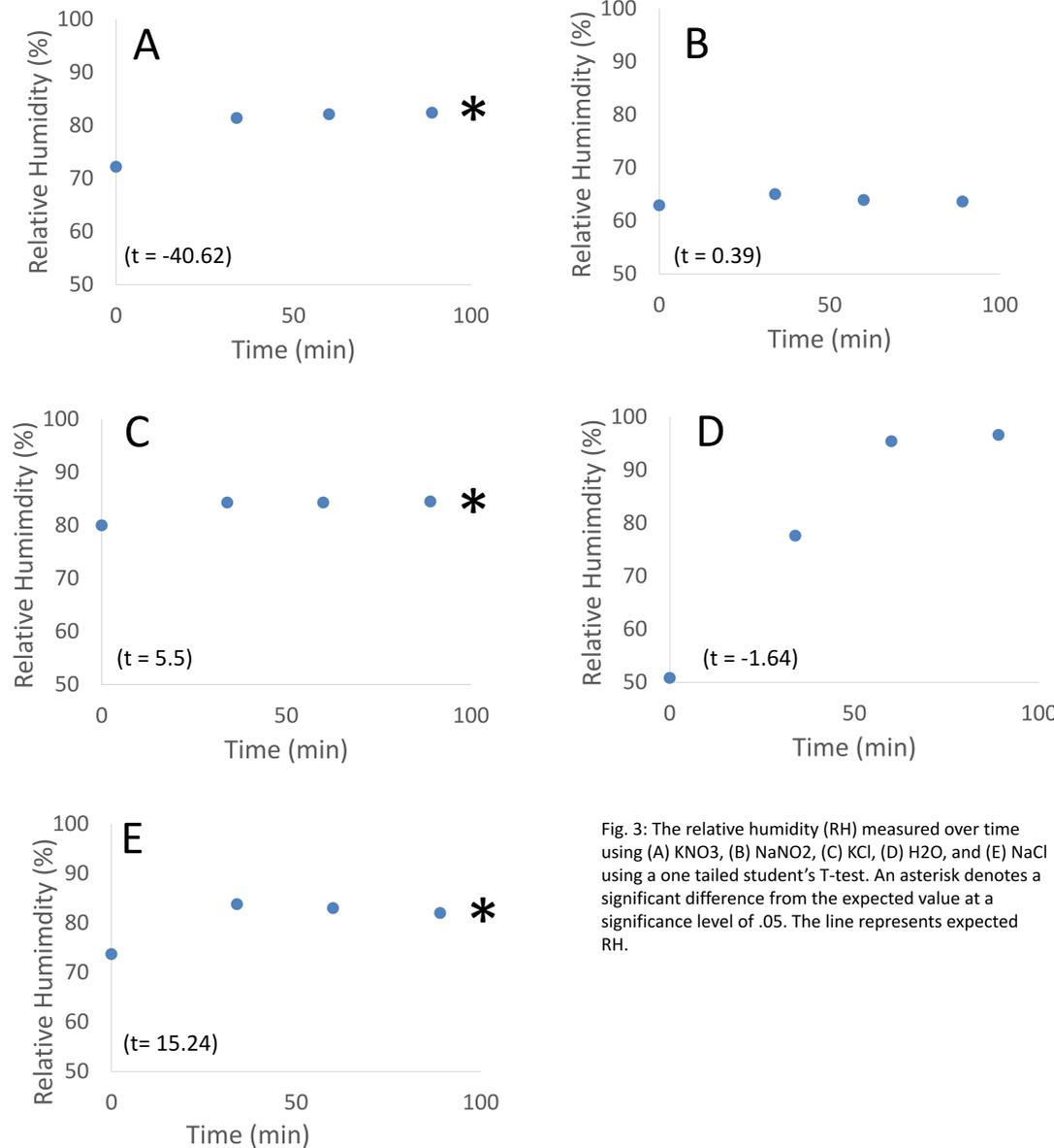
Fig. 3: The relative humidity (RH) measured over time using (A) KNO<sub>3</sub>, (B) NaNO<sub>2</sub>, (C) KCl, (D) H<sub>2</sub>O, and (E) NaCl using a one tailed student's T-test. An asterisk denotes a significant difference from the expected value at a significance level of .05. The line represents expected RH.
