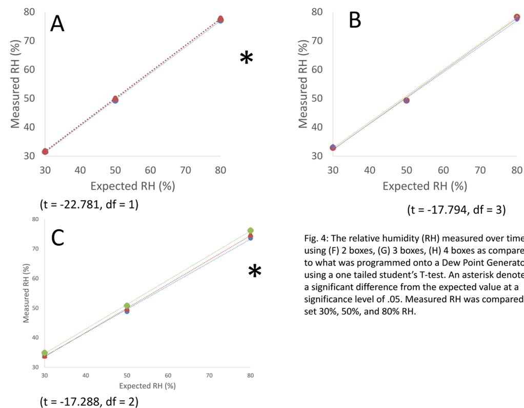
Fig. 4: The relative humidity (RH) measured over time using (F) 2 boxes, (G) 3 boxes, (H) 4 boxes as compared to what was programmed onto a Dew Point Generator, using a one tailed student's T-test. An asterisk denotes a significant difference from the expected value at a significance level of .05. Measured RH was compared to set 30%, 50%, and 80% RH.
