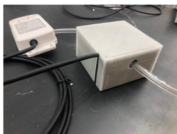
Fig. 2: Gametophyte Chamber attached to a HOBOT sensor and tubing. The HOBOT sensor continuously measured temperature and relative humidity inside the chamber throughout the experiments.
