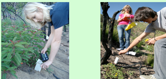
Fig. 2 A Hydrosense Soil Water Measurement System was used to measure the percent volumetric water content at predawn and dusk for six specimens of both Ceanothus megacarpus and Malosma laurina . Four readings were taken for each plant with corresponding controls.
